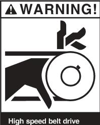
Aligh speed belt drive operating overhead. Can cause serious injury. Keep head and hands clear. Do not enter when dryer is running.
