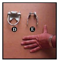
Photo B-8 D. 1-1/2" Korn Clamp. E. 1-1/2" Strut Clamp. (Use 1/2" to 2-1/2".)
