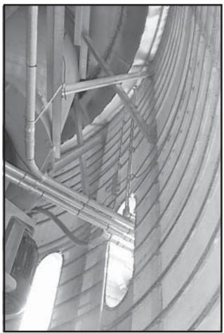
*Photo 2-19 RH view - Fan Motors wired and Air Switch Tubing installed.*
