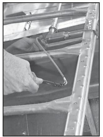
Photo 1-35 Pulling wires to Exterior Hi-Limits.
