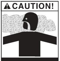
Airborne particles during operation. May impair vision and breathing. Do not enter when dryer is running.
