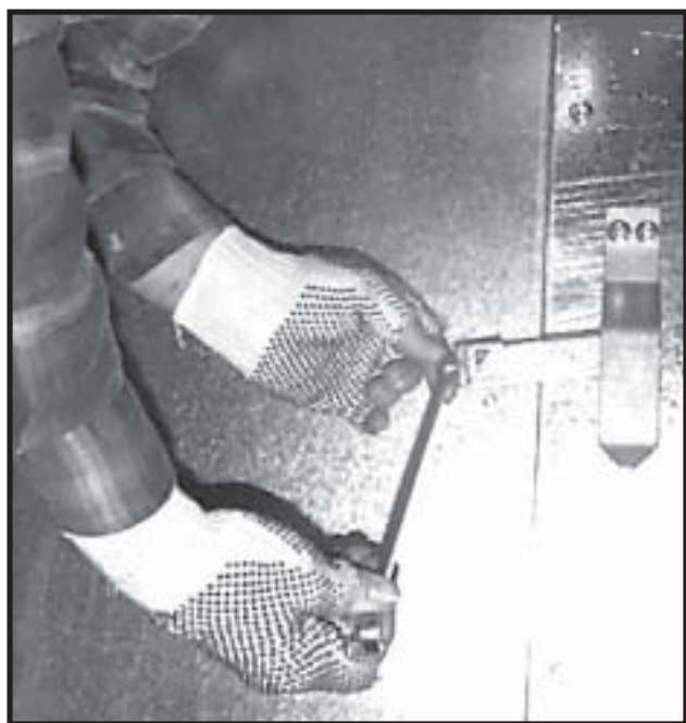
Photo 16-50 Adjusting bolt on Latch Bar.
