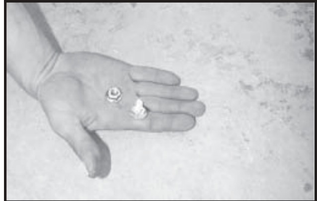
Photo 16-3 5/16" x 3/4" Slotted Truss Head bolt and 5/16" Whiz Lock nut.
