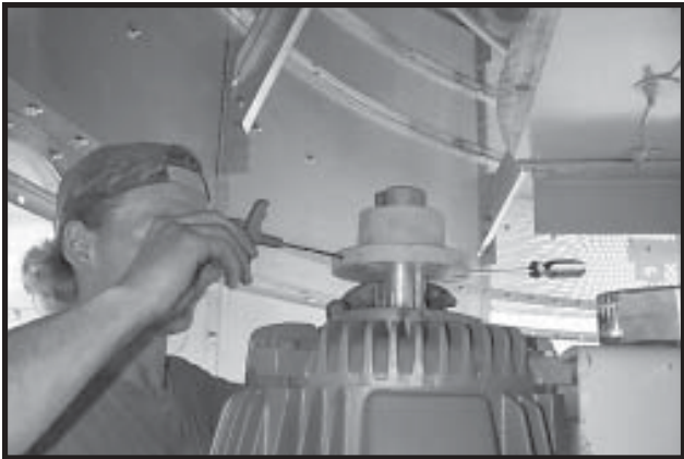
Photo 14-15 Tightening set screw on Motor Hub.
