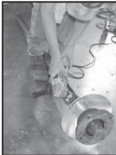
Photo 20-15 Cleaning Metering Drum Drive Shaft Weldment.
