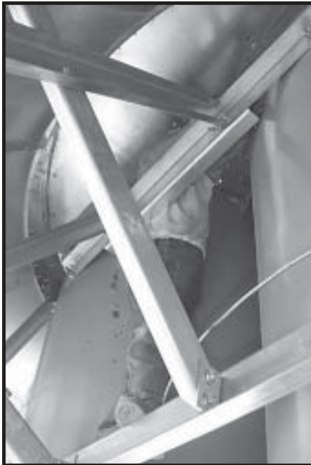
Photo 15-5 Accessing upper Grease Zert.
