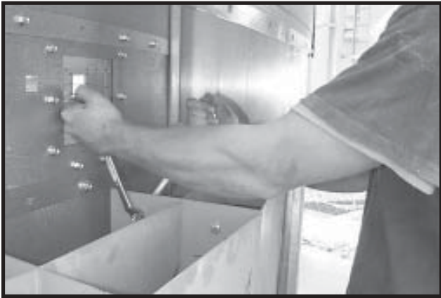
Photo 11-5 Tightening Grain Turner Sections.
