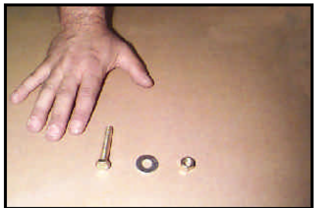
Photo B-14 3/8" x 2" Bolt, washer & nut.
