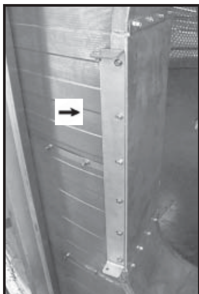
Photo 16-33 Use common bolts on Latch/Hinge Bracket, Window Frame, and Outside Wall Sheets (arrow). Insert bolts toward inside of dryer.
