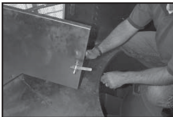
Photo 16-53 Reducer Door is installed. Note hinges are on LH side in this example.
