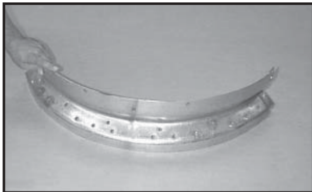
Photo 3-12 Tower Roof Center Collar Section (1 of 3).
