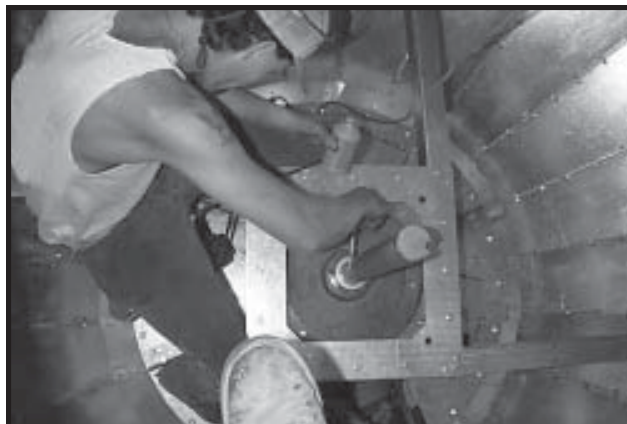
Photo 20-23 Applying anti-seize to Metering Drum Drive Shaft.
