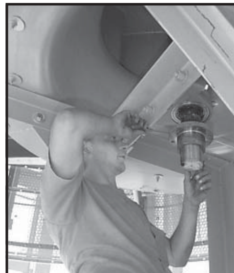
Photo 14-20 Tightening set screw on Fan Hub.
