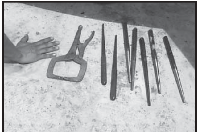
Photo 2-12 C-Clamp and Alignment Punches (5/8" & larger).
