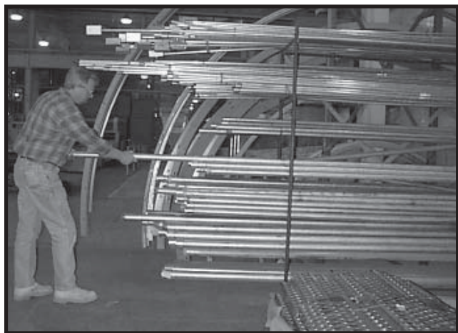
Photo 5-1 1/2" IMC rigid, threaded conduit.
