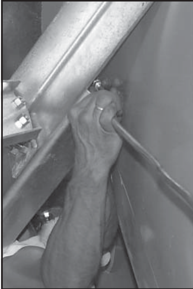
Photo 15-10 Attaching Grease Tube to Brass Compression Union.
