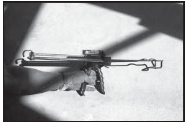
Photo 17-27 Ceramic Epoxy Injection Tool.
