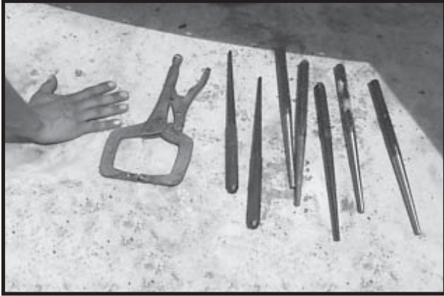
Photo A-1 C-clamp and assorted alignment punches.
