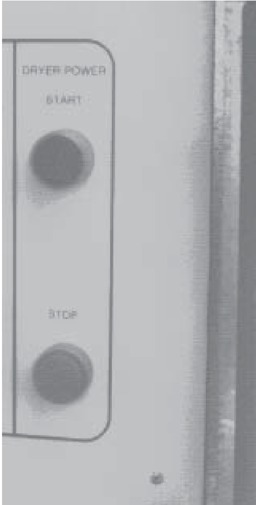
The lighted start switch indicates that the dryer is operational.
