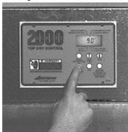
Set grain temperature on control panel display.
