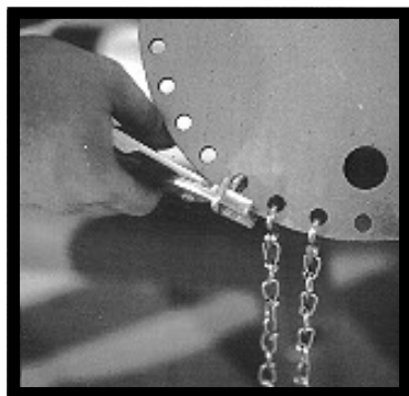
Crimp "S" hooks after final chute adjustment
