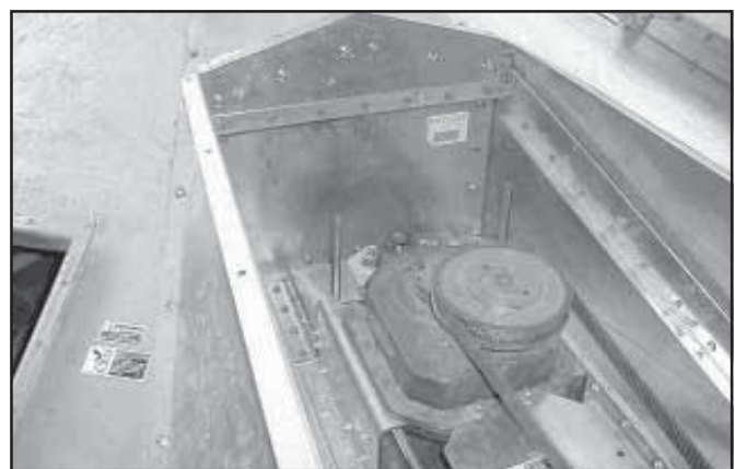
11-C. Assembled Drive with Weather Guard Components.
