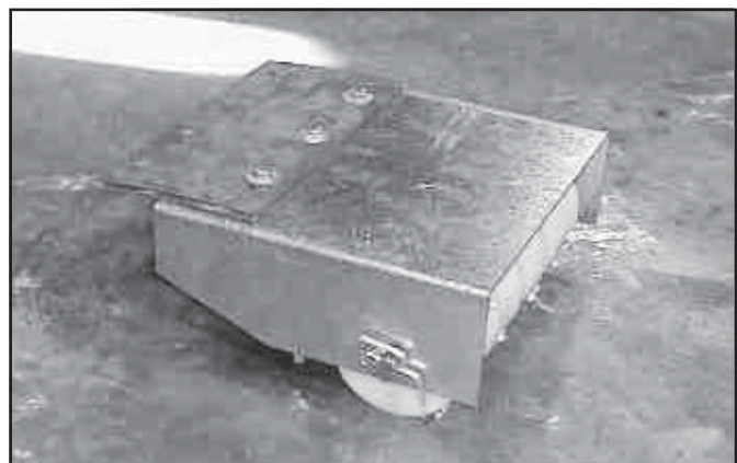
9-G. Close-up of Cleaning Roller.
