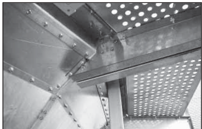
8-B. Platform Support Channels. RMS 15K Shown.
