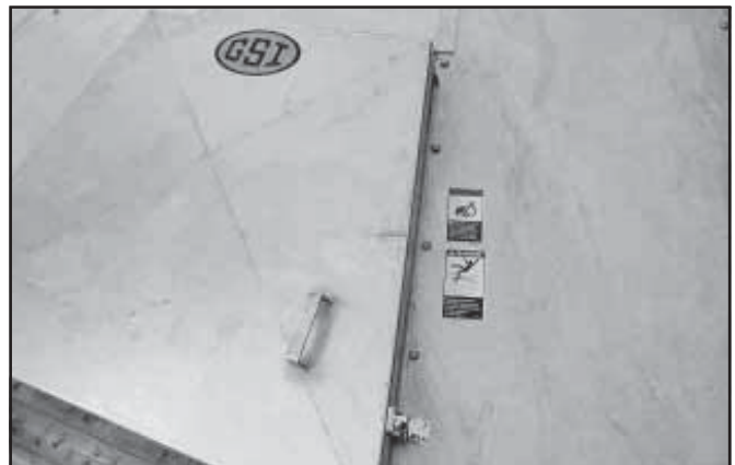
10-G. Access Door with Latch and Safety Labels.
