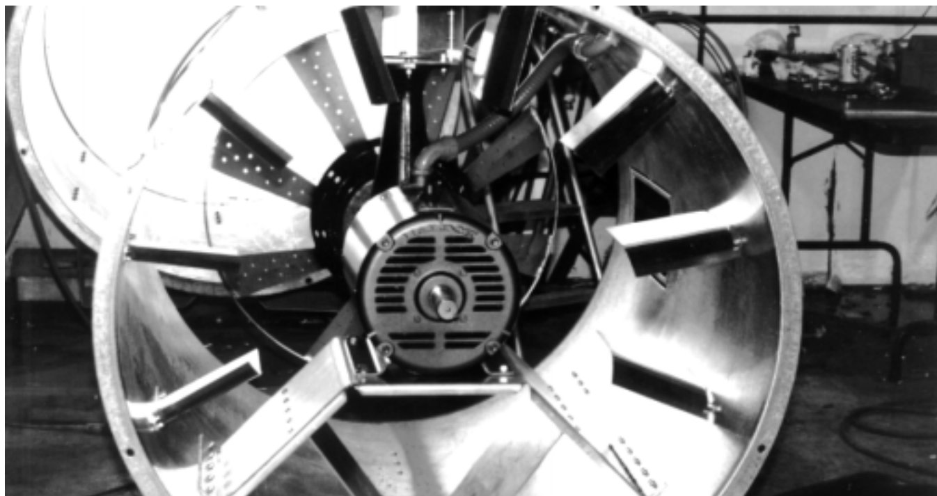
The position of the fan motor provides easy access for service.
