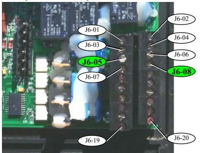
\*\*The J6 terminal strips are two strips with ten terminals on each strip. The left strip is the odd numbered J6 terminals (i.e. J6-01, J6-03,... J6-19). The right strip is the even numbered J6 terminals (i.e. J6-02, J6-04,... J6-20).
