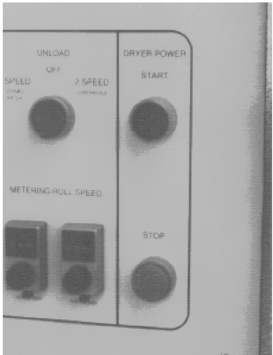
The lighted start switch indicates that the dryer is operational.
