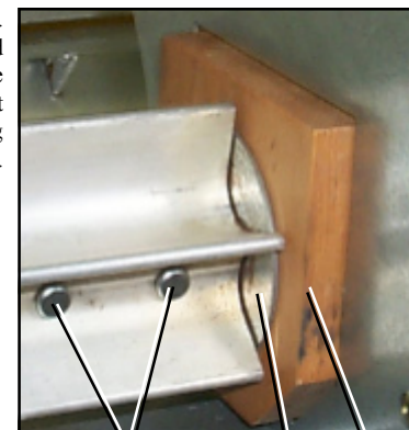
Wooden meter roll support bearing. The meter roll sections are spliced together with a meter roll splice shaft (part no. D31-0046) that passes through the support bearing assembly.
