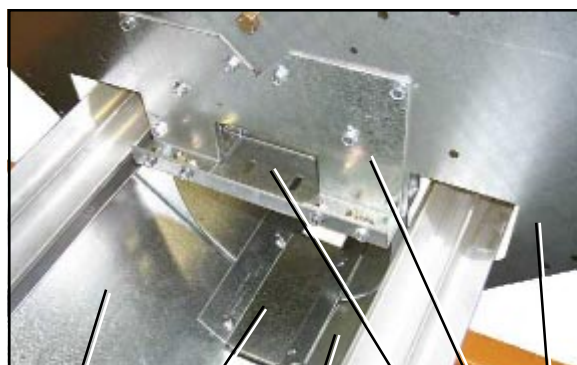
Center hanger bearing support and cross channel seal plate.
