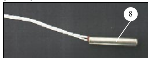
Grain temperature thermister. There are 2 thermisters in each (right & left) grain high limit thermostat assemblies.
