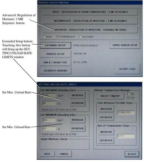
9. You should now be back in the Moisture Control Selection window. Touch the BIN #/GRAIN TYPE button. When the Storage Parameters window appears select the type of grain that is to be dried and select the storage bin to be used (the bin
