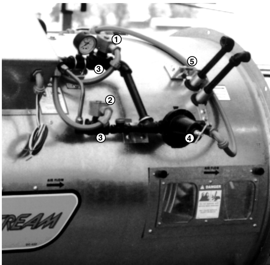
This view of the dryer heater shows 1-high pressure gas solenoid, 2-low pressure gas solenoid, 3-gas solenoid valves, 4-gas regulator and 5-vaporizer adjustment bracket
