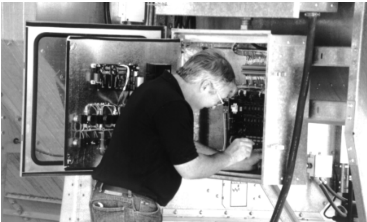
Airstream Service Technician checks the wiring on a dryer control box.
