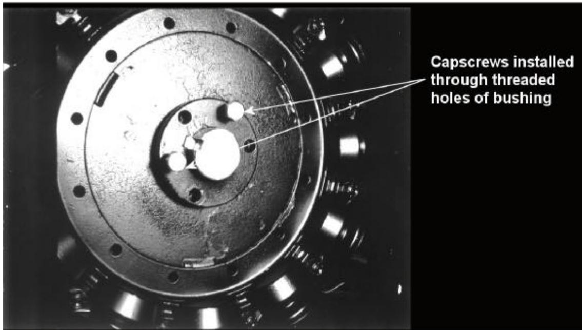
3. Install two of the cap screws into the threaded holes in bushing, and turn them by hand until they bottom against the front surface of the blade. **NOTE:** The threaded holes within the bushing are provided for disassembly purposes only. Do not attempt to use these holes for reassembly. They will not allow the parts to lock onto the shaft thereby causing a hazardous operating condition.
