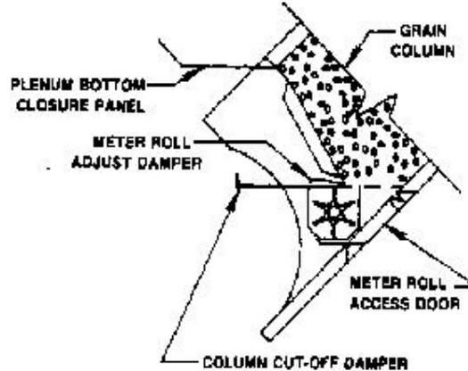
This column cutoff damper is designed to insert through the grain column (from the inside of the dryer) immediately above the metering roll. This permits opening of the metering roll access door. For service or inspection without unloading the dryer, the plenum bottom closure panel and metering roll adjust damper must be removed prior to using service tool.
