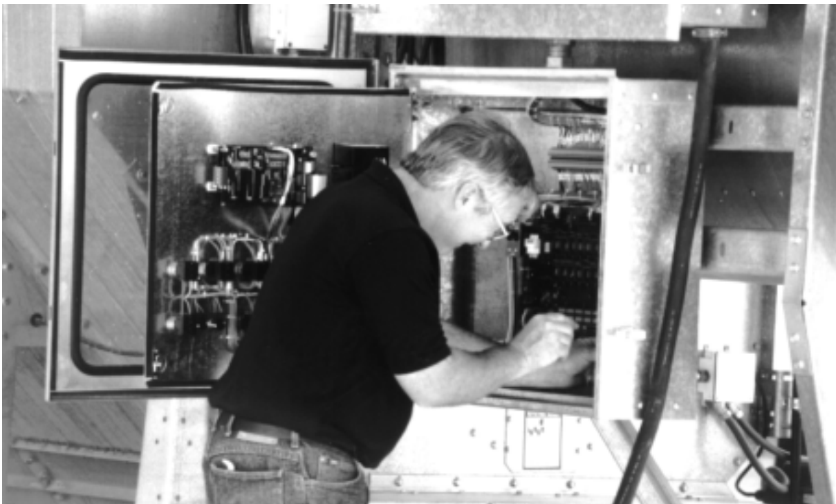
Airstream Service Technician checks the wiring on a grain dryer control panel.
