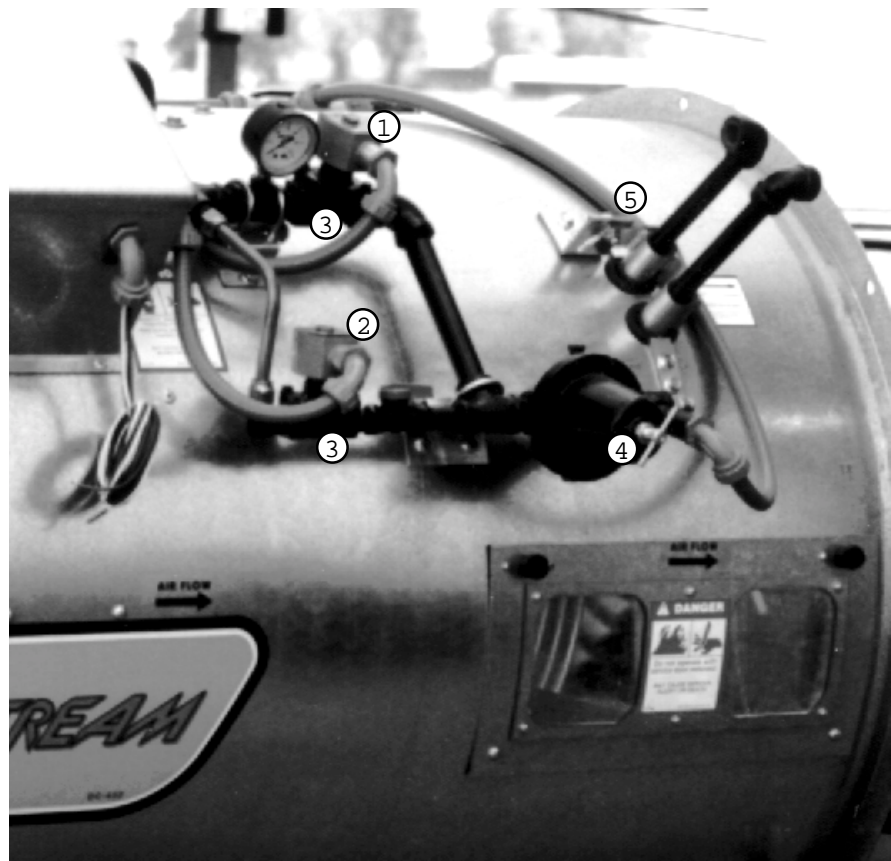
This view of the dryer heater shows 1-high pressure gas solenoid, 2-low pressure gas solenoid, 3-gas solenoid valves, 4-gas regulator and 5-vaporizer adjustment bracket
