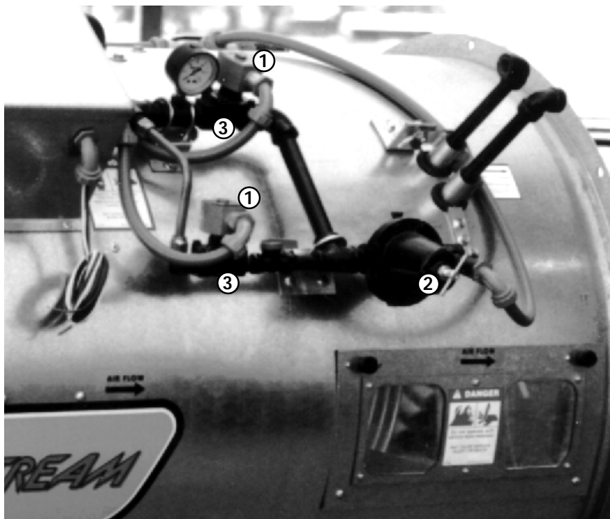
This view of the dryer heater shows 1-gas solenoid valve coils and 2-gas regulator and 3-gas solenoid valves.
