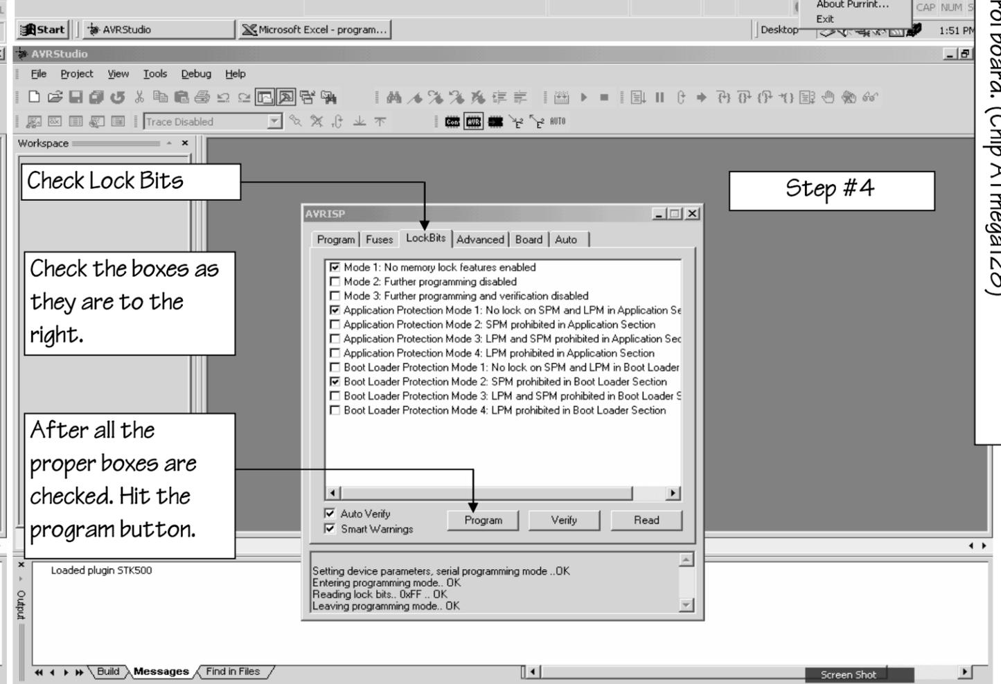
The following are instructions on how to load the bootloader to the moisture control board. (Chip ATmega128)
