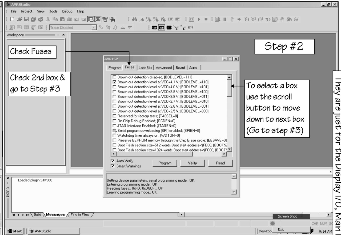
The following instructions are for loading the bootloader to each individual board. They are just for the Display I/O, Main I/O & F/H Boards ( Chip AT90CAN128 )
