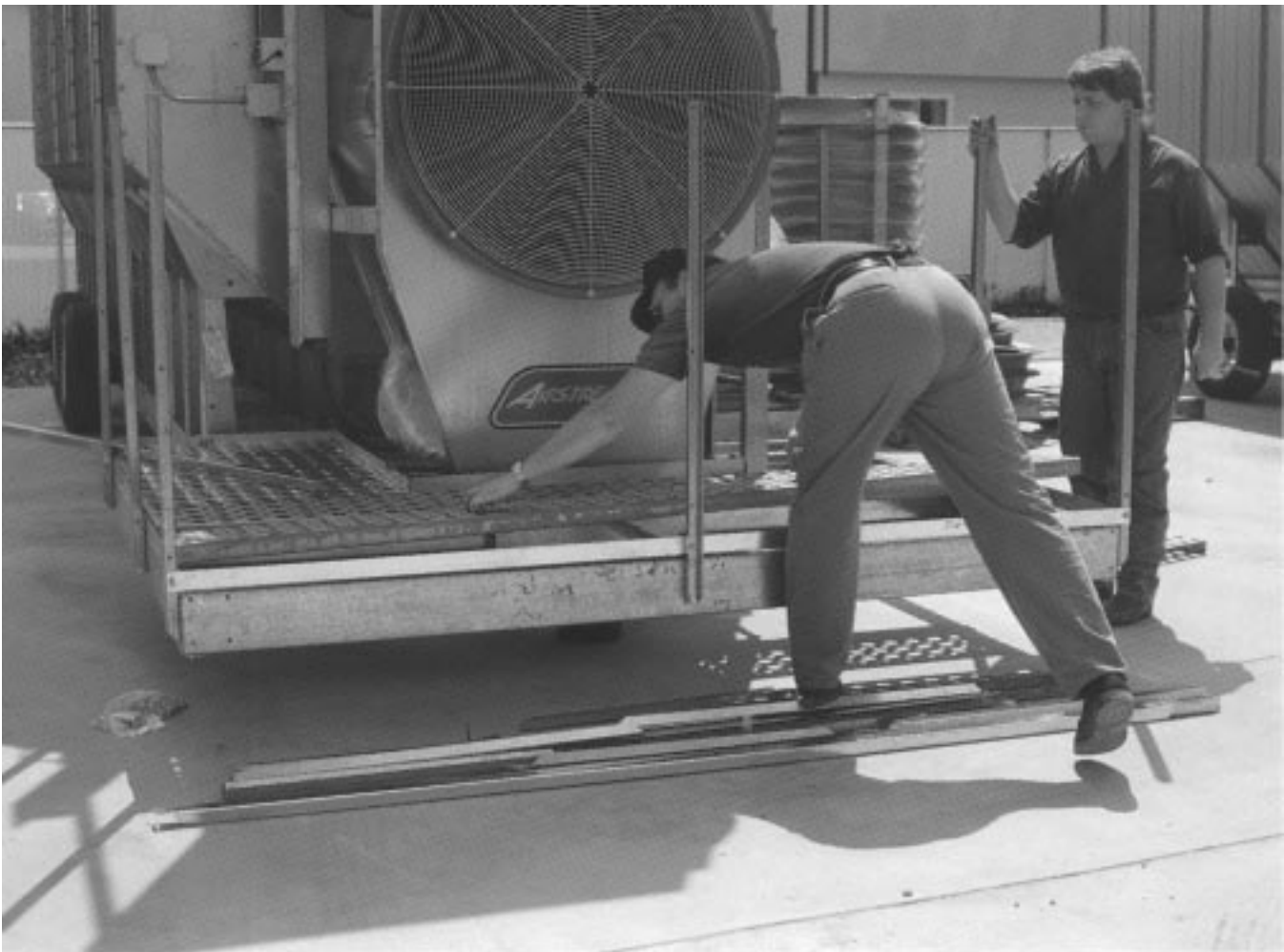
Figure 18: Installing center long floor panels.
