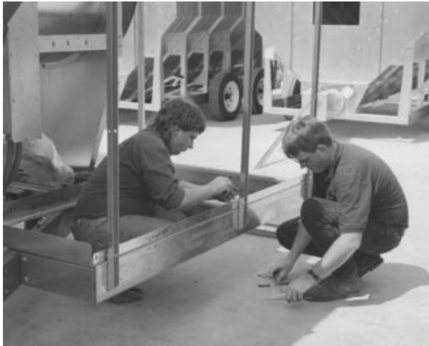
Figure 15: Connecting outer front toe board to guard rail support channels.
