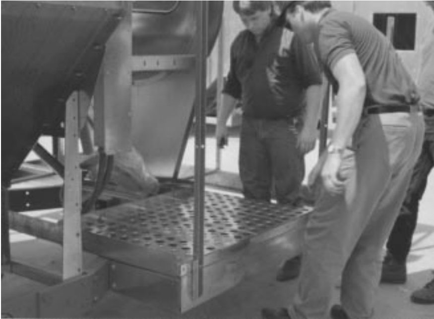
Figure 17: Installing four short floor panels.
