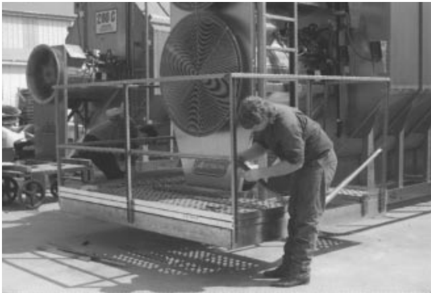
Figure 22, top: Installing front and side upper guard rails. Figure 23, above: Installing lower side guard rails. Figure 24, right: Installing lower rear guard rail.
