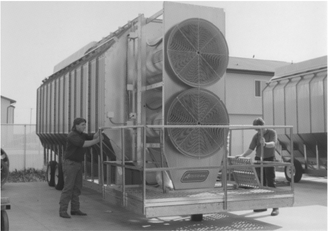
Figure 28: Check to make sure every bolt is tight and door opens freely.
