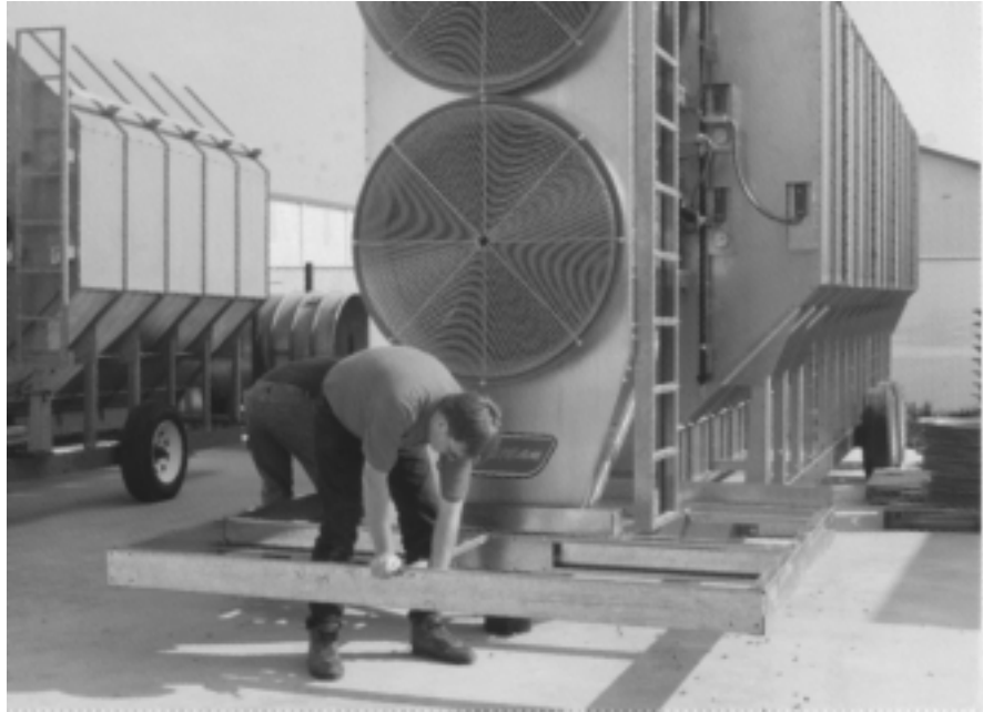
Figure 9: Center floor support placement.
