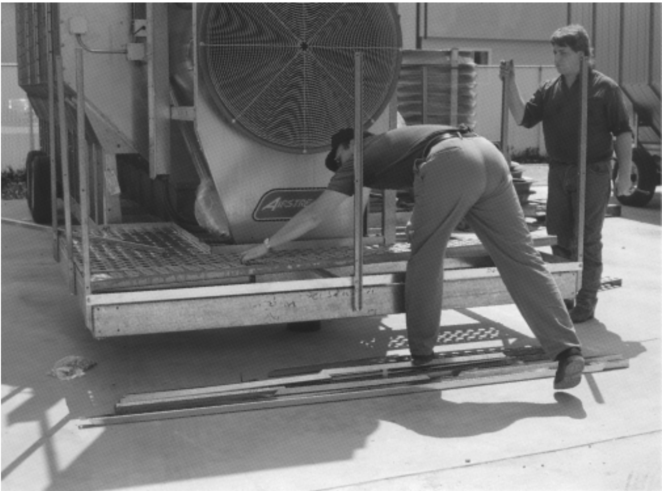
Figure 18: Installing center long floor panels.
