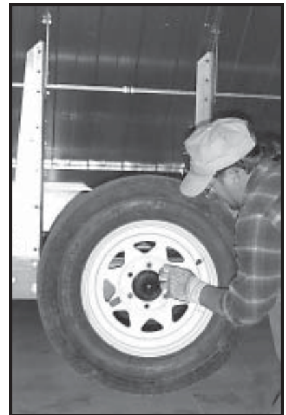
Photo 10-12 Putting lug nuts on transport single wheel assembly.
