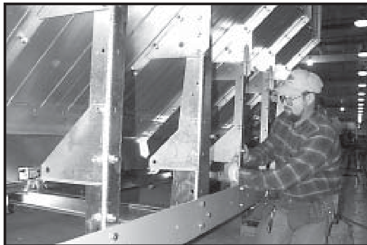
Photo 9-6 Bolting pivot rod bracket to side leg in front of center leg.
