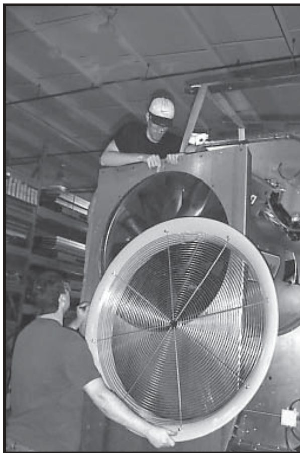
Photo 18-55 Loosely bolting venturi through front fan support to fan-end of fan-heater assembly.
