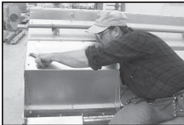
Photo 21-14 Bolting LH wet bin end section to wet bin end on top auger housing assembly.
