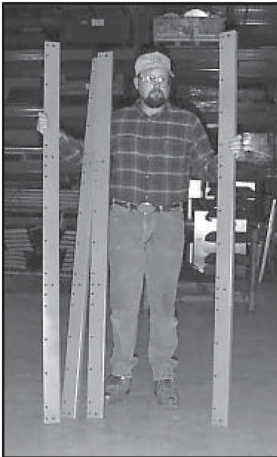
Photo 7-2 Top edge angles-P (painted) for installation along sides of dryer. Top edge angles are shipped painted.
