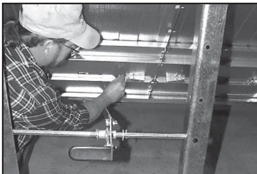
Photo 24-3 Inserting meter roll door latch through ears on trough panel weldment and securing with hairpin.
