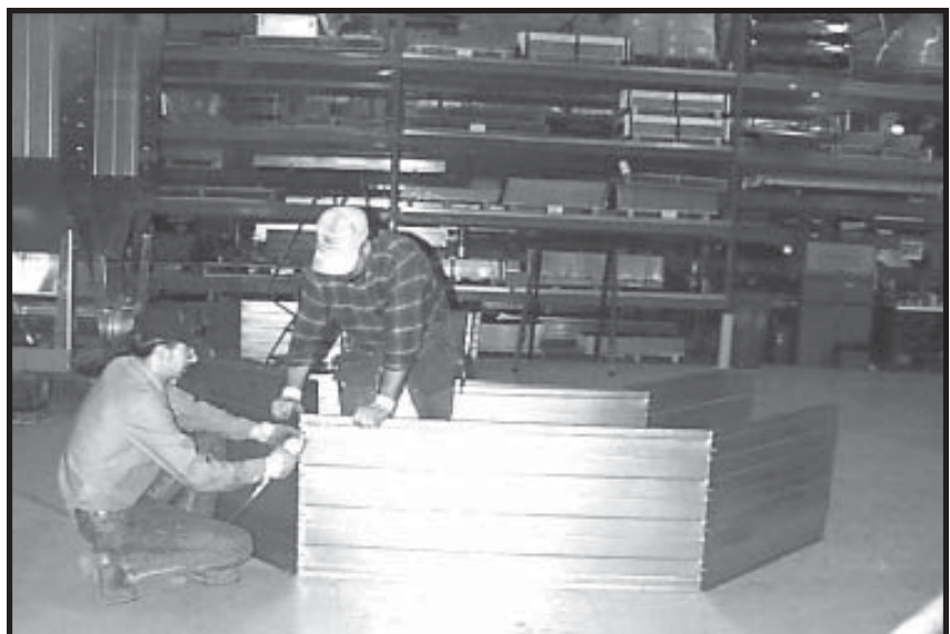
Photo 6-2 Assembling hopper sheet, to outside wall, to roof sheet.
