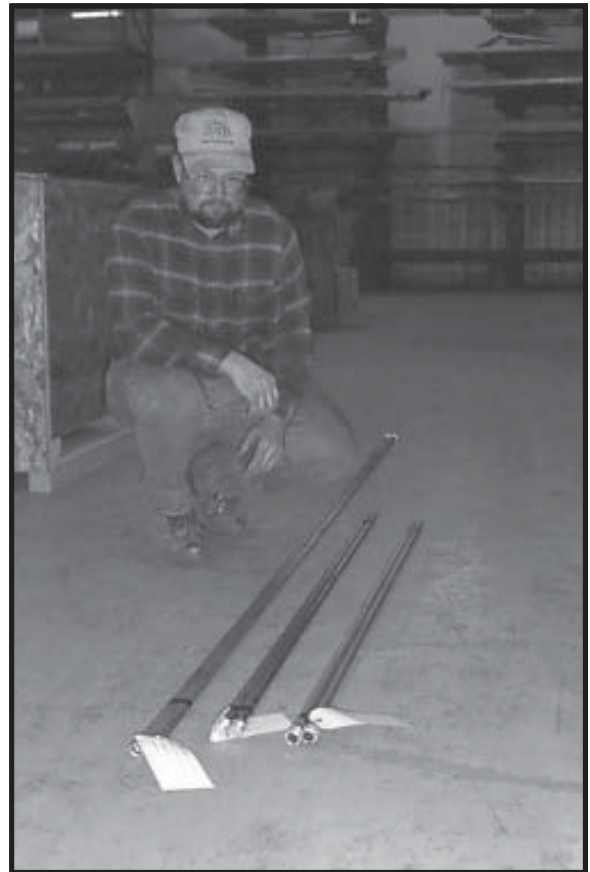
Photo 5-1 EMT conduit, column hi-limit for 22' dryer.
