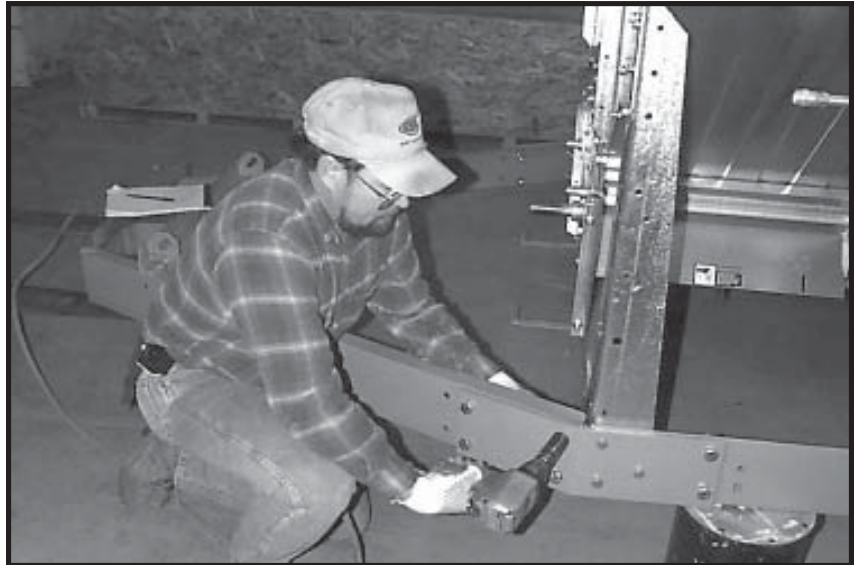
Photo 14-4 Bolting LH side of hitch weldment to LH hitch bracket.
