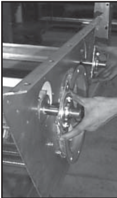
Photo 2-39 Sliding 1" meter roll bearing assembly on meter roll assembly stub shafts at (rear) discharge bearing plate.
