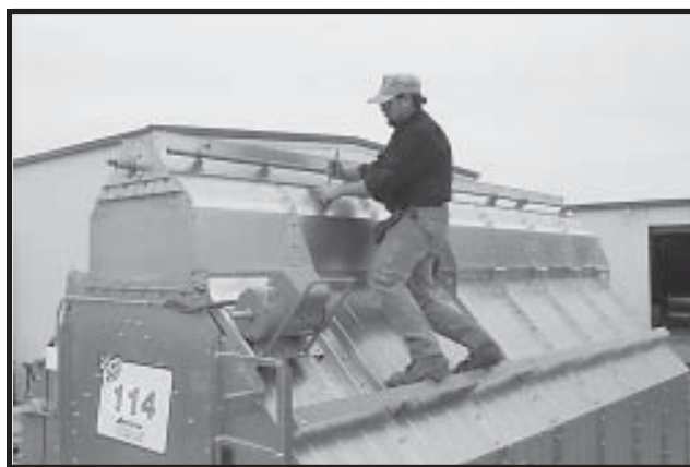
Photo 21-16 Aligning holes in wet bin section to top auger housing assembly.
