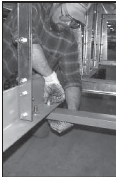
Photo 10-11 Loosely bolting axle cross channel in center hole of RH and LH transport single wheel assembly.
