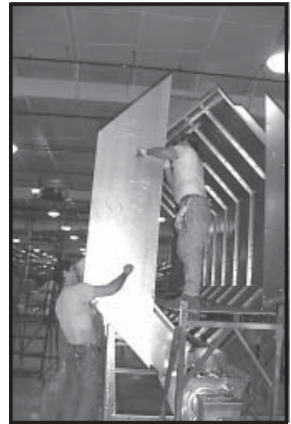
Photo 3-43 Lifting LH rear column end panel into place using 3/8" punches.
