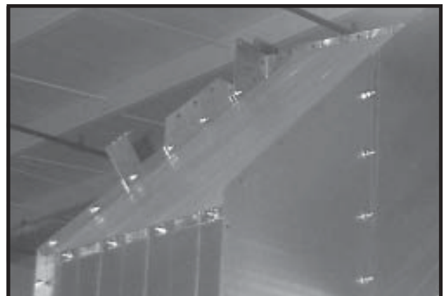
Photo 6-7 First set of brackets bolted in LH front of dryer.
