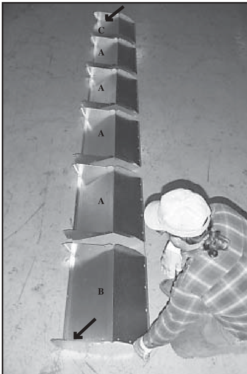
Photo 17-1 Placement of wet bin sides (galvanized, perforated) as they will be installed to dryer. (RH rear view or LH front view)
