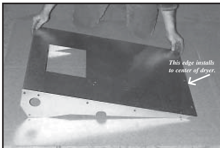
Photo 4-1 Bottom plenum divider end installs at front LH and rear RH of dryer.
