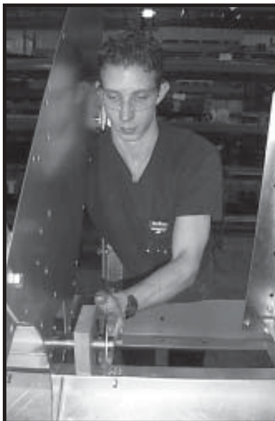
Photo 2-33 Sliding washer, wooden bearing, and second washer onto splice shaft of front meter roll assembly.
