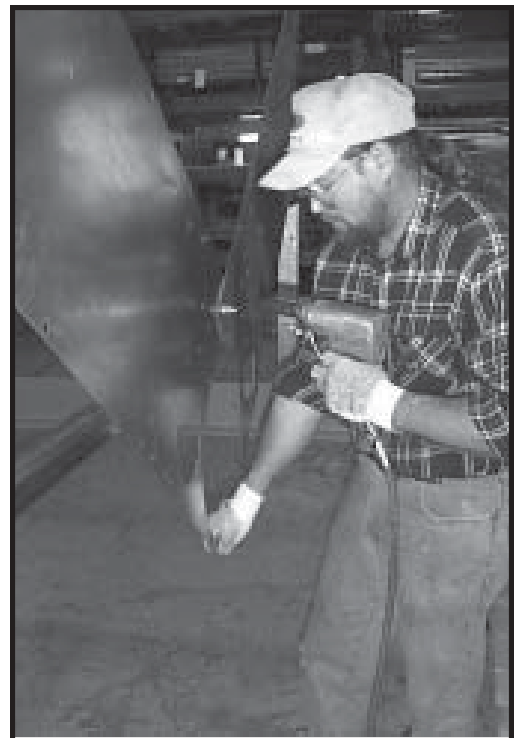
Photo 2-14 Tightening bolts with approximately 4" gap between bulkheads at lowest point.
