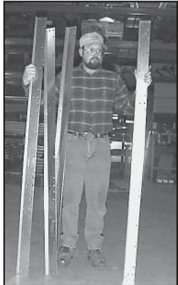
Photo 7-1 Top edge angles (unpainted) for installation at top of dryer.
