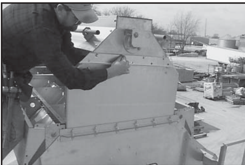
Photo 21-13 Rear view - installing auger housing end tie channel.
