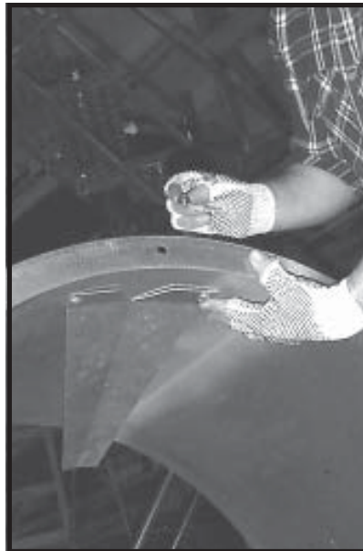
Photo 11-4 Installing airmixer vanes on air mixer can.
