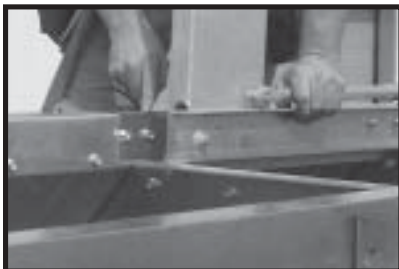
Photo 20-2 Front of lift kit aligned to RH splice on RH top edge angle.
