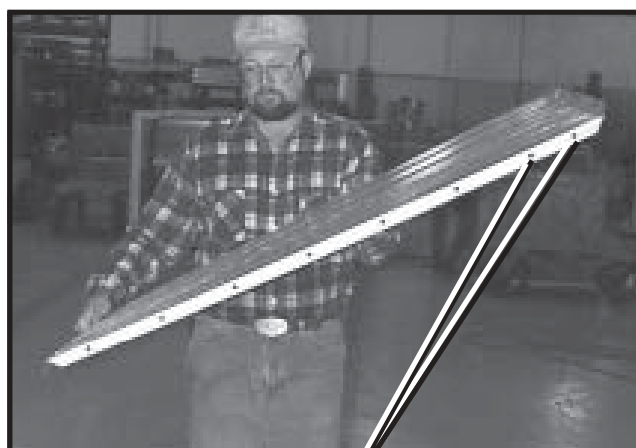
Photo 3-32 Top of plenum top has (2) closely spaced holes.
