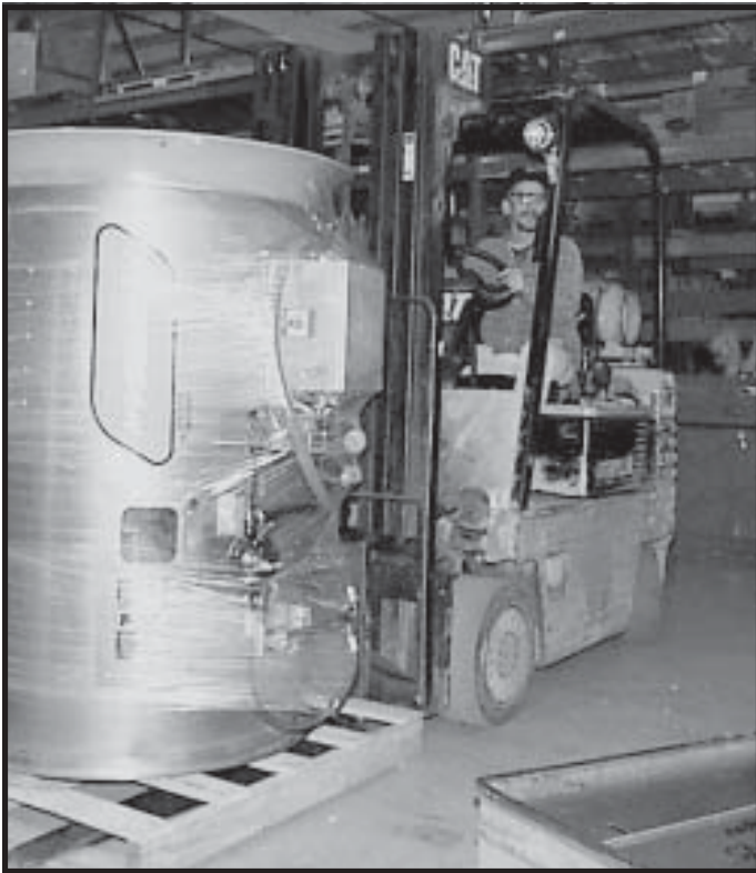
Photo 1-1 Fan/heater unit as shipped (inverted on shipping pallet).
