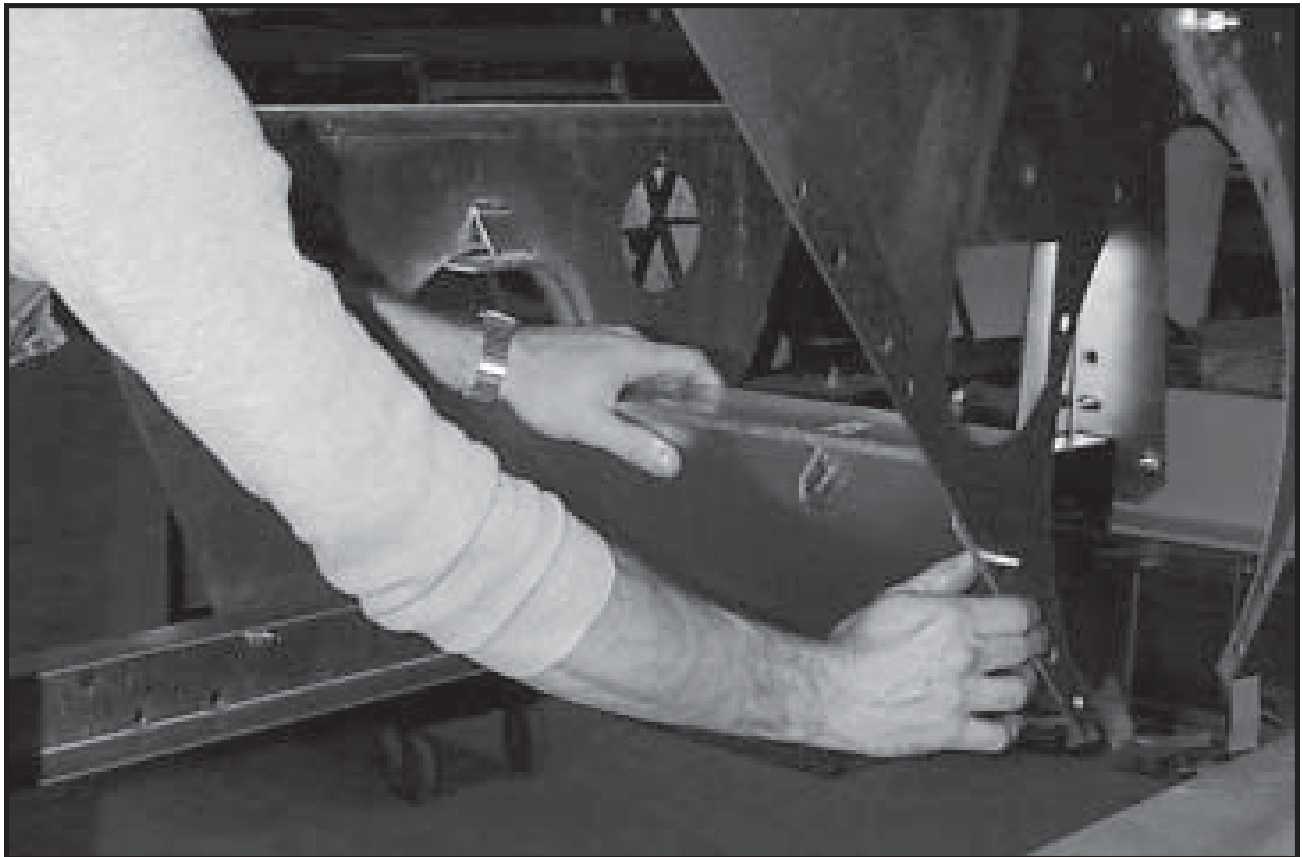
Photo 2-18 Loosely bolting rear trough panel weldment to discharge bearing plate.
