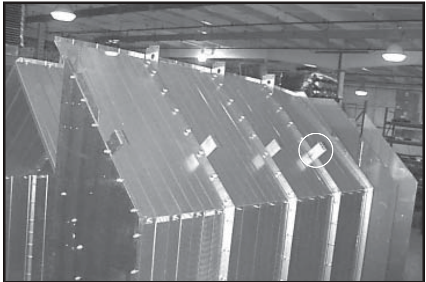
Photo 6-10 Brackets and outside screen installed in LH side of dryer. Note (2) walk rail brackets (circled in photo), one on each side of seam above frame tie channels.
