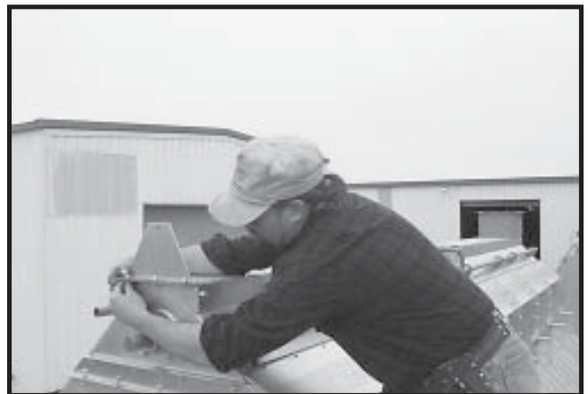
Photo 23-4 Bolting belt guard mounting bracket to top auger housing assembly.
