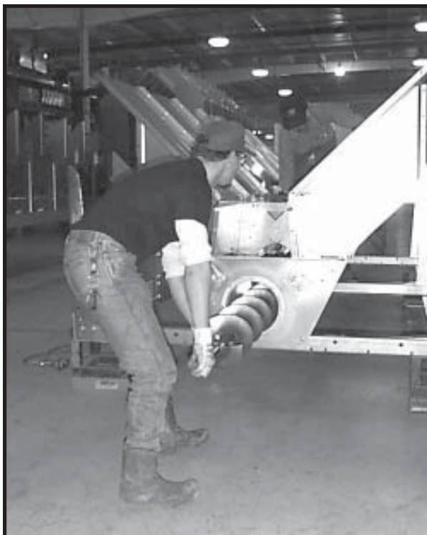
Photo 3-20 Inserting rear auger section of bottom rear auger weldment.
