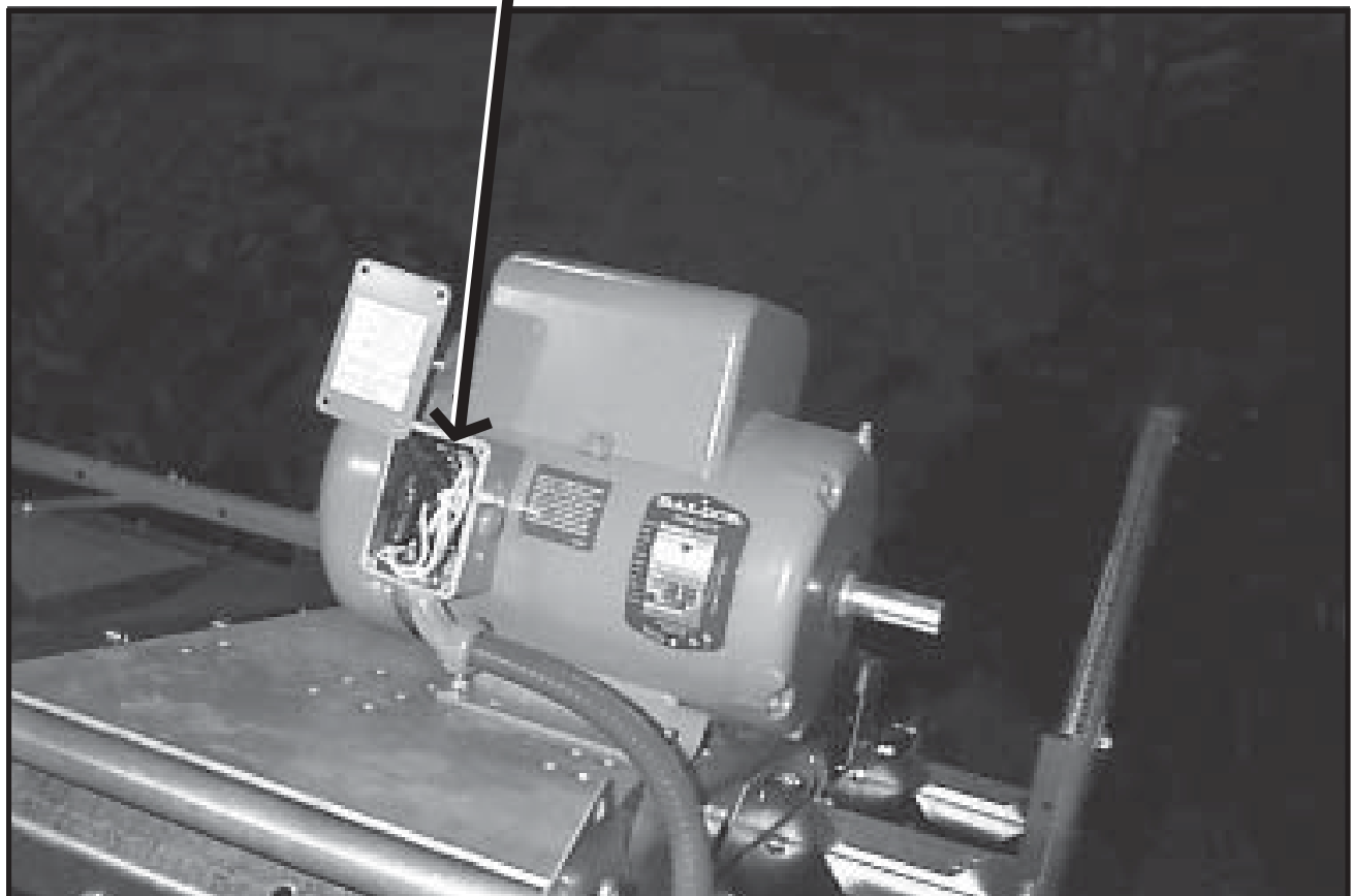
Photo 18-43 Load motor wired, with name plate lifted.
