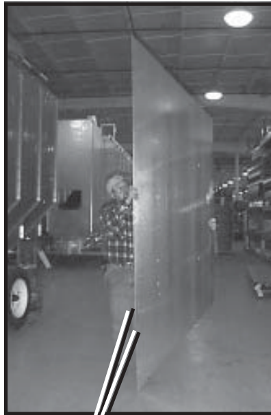
Photo 3-42 Bottom edge of column end panel has two large notches on longest edge.
