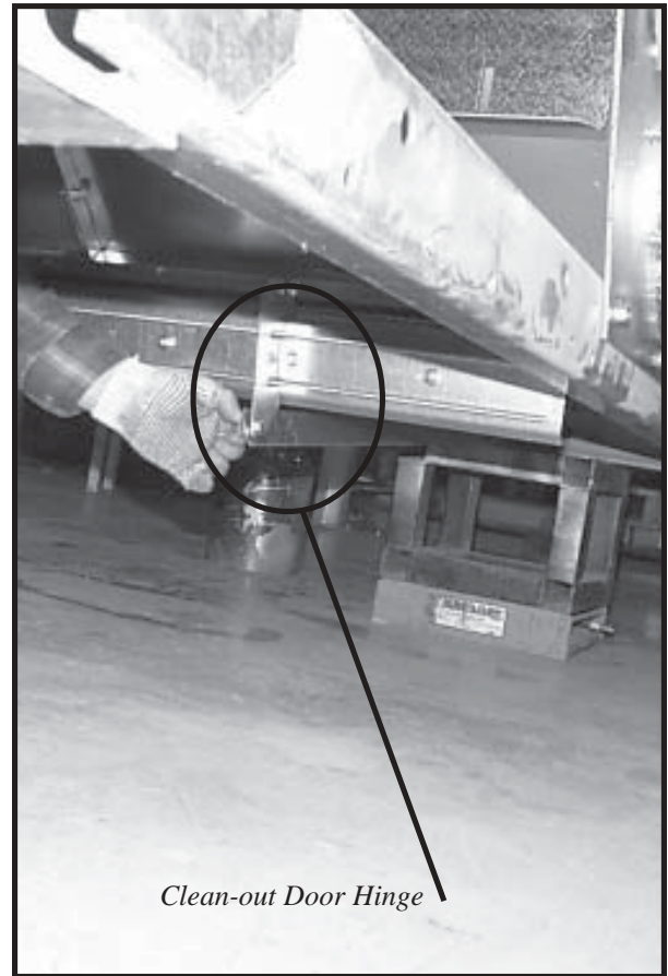
Photo 9-12 Linkage bar bolted to clean-out door assembly. (view from rear LH side of dryer)
