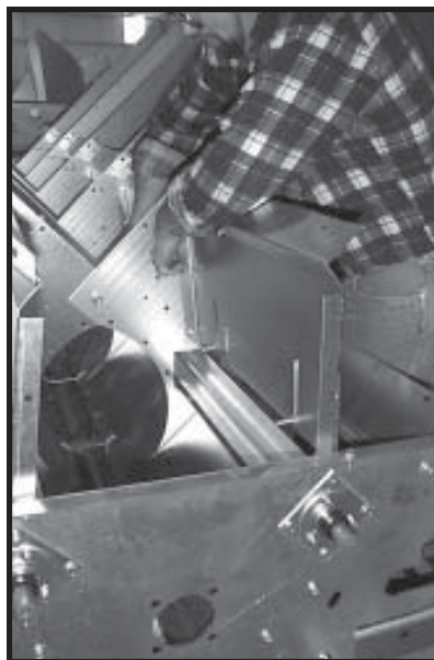
Photo 2-48 Bolting (2) meter roll upper shield assemblies on hopper bulkhead.
