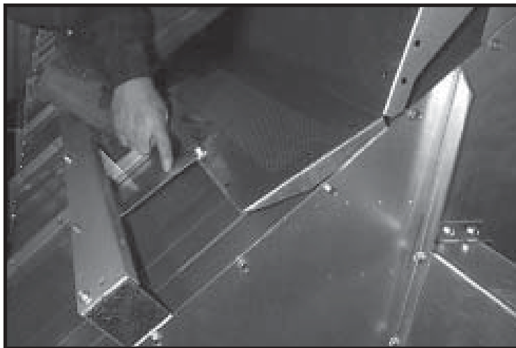
Photo 17-7 Wet bins folded down and brackets (tie-downs) installed.
