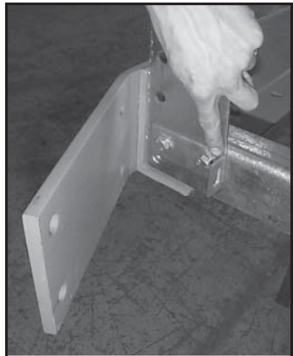
Photo 2-7 Slotted hole on motor mount adjustment bracket.
