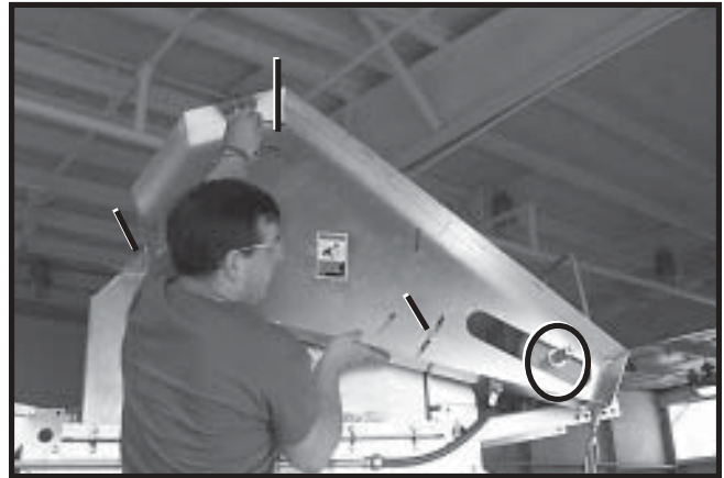
Photo 23-11 Placing top auger belt guard body over (3) bolts (arrows), with cutout centered on load motor drive shaft (circle.)
