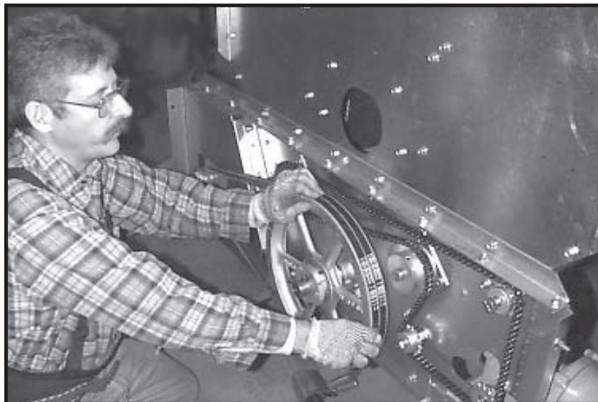
Photo 15-22 Installing belts on auger pulley.
