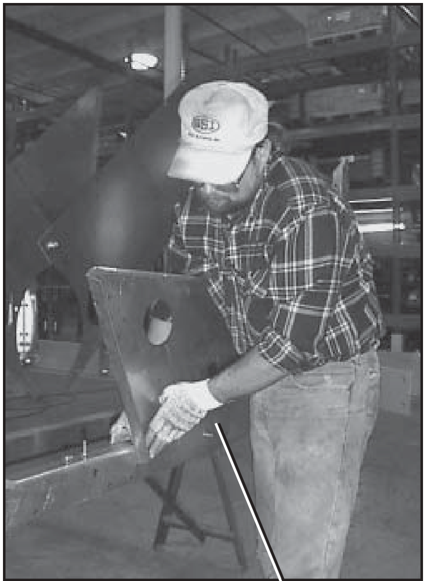
Photo 2-15 Positioning auger bearing plate. (front of dryer)
