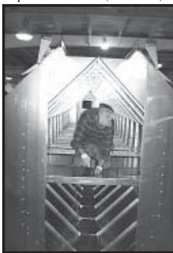
Photo 4-26 Tightening screws in previous pair of plenum sheets.
