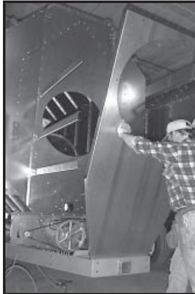
Photo 16-6 Lifting front fan support onto hitch weldment.
