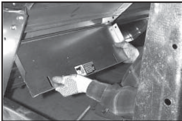
Photo 8-2 Placing access door between hopper bulk-heads in first holes beneath connector sheet.
