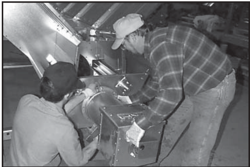
Photo 3-23 Placing discharge auger assembly over bottom rear auger weldment.
