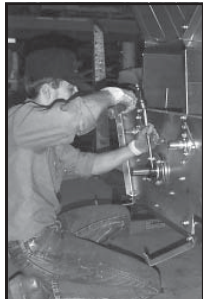
Photo 3-18 Loosely bolting flangette bearing to bottom auger bearing plate.
