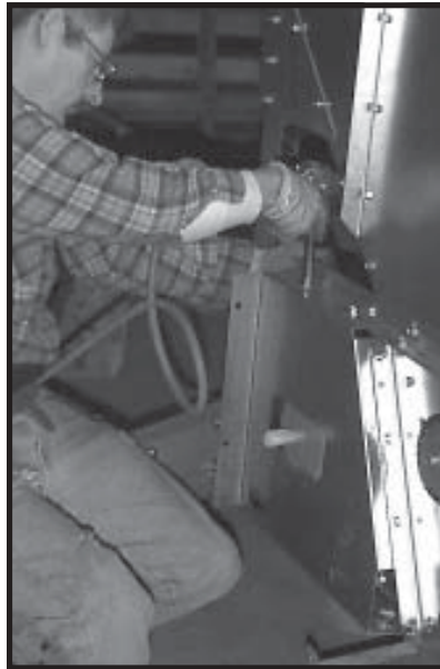
Photo 15-18 Tightening belt guard on unload motor.
