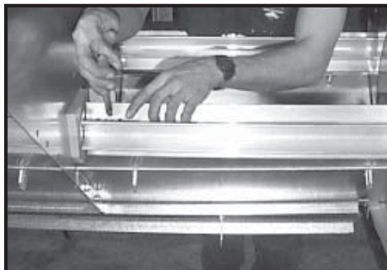
Photo 2-36 Bending cotter pins through clevis pins.
