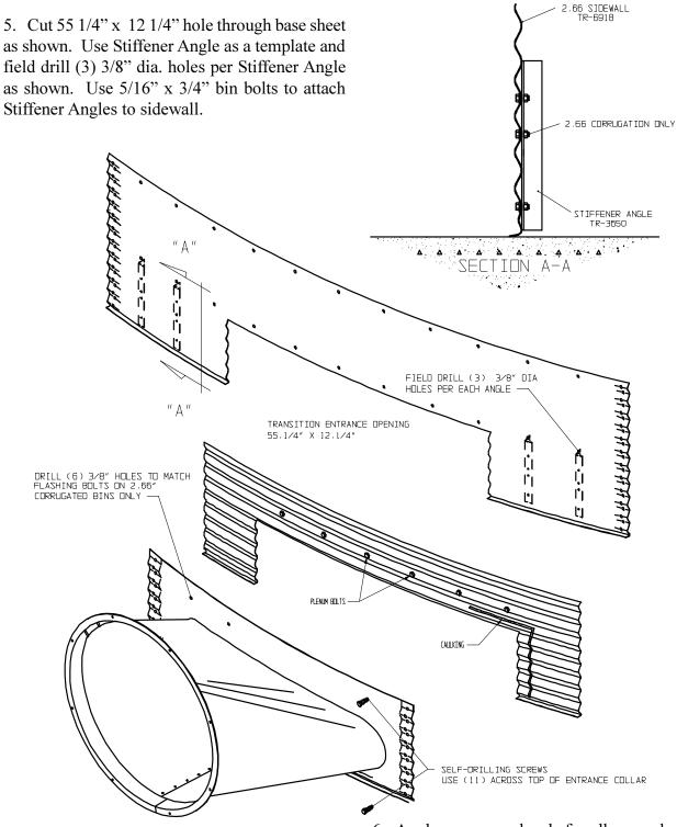
6. Apply a generous bead of caulk around perimeter of opening. Using self-drilling screws attach Transition Housing Assembly as shown.
