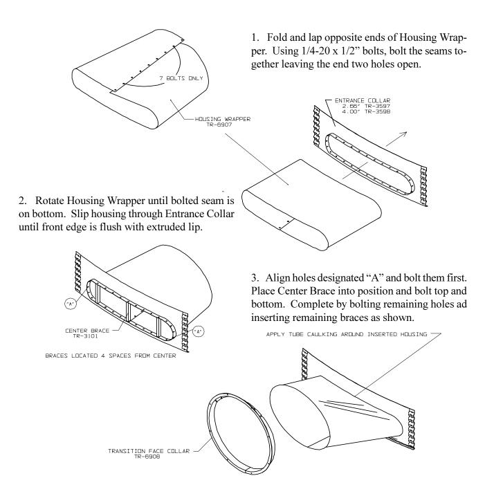
4. Slide Transition Face Collar into opening, with crimped surface at top. Secure with remaining bolts.
