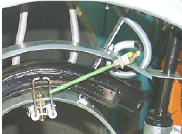
Figure 1. Flame Switch should be mounted so it lies across the burner. Try to keep the switch in a position where the flame will cover the middle portion of the ceramic coating.
