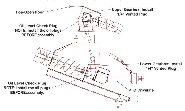
**NOTE:** The Upper Gearbox is filled with oil at the factory. The Lower Gearbox is shipped without oil.
